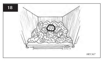
8.11 Place two small coals to the left and right-hand side of the bed in the two remaining spaces, Diagram 19.
